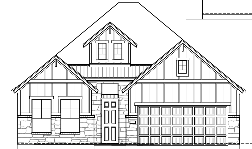
FRONT ELEVATION 'A2' STONE OPTION
