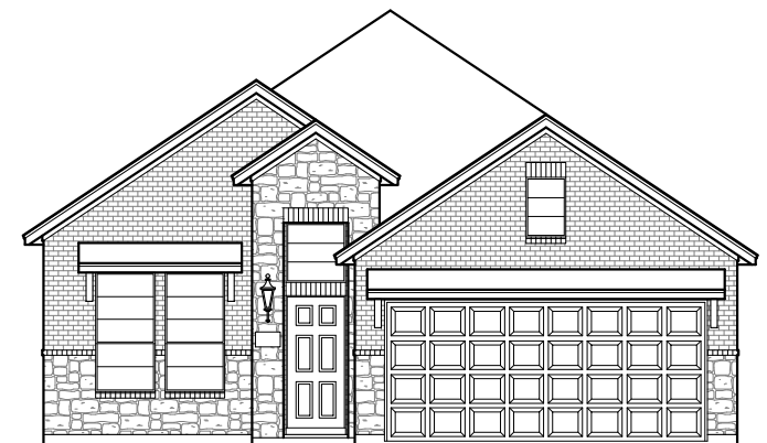
FRONT ELEVATION 'A1' BRICK & STONE OPTION
